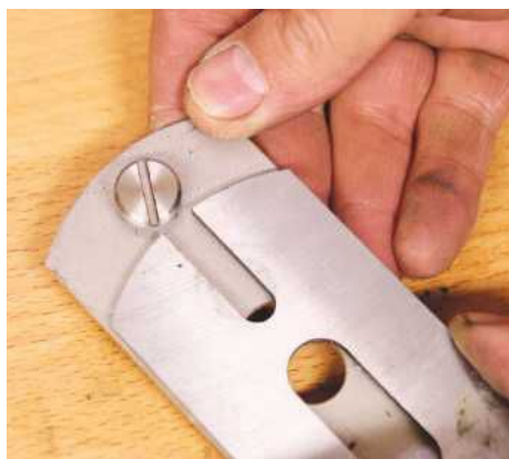
▲ The double irons connect together with a screw through a slot
